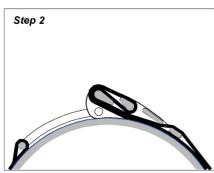
Rotate the cam closed. It should require a fair amount of force, but do not overtension. Ask a dive professional if you are not sure of the correct tightness. Aggressive jerking on the harness can test for secure assembly. Do not get body parts caught in the cam, it can cause serious injury. Secure the end of the webbing with Velcro or lace through a keeper.
