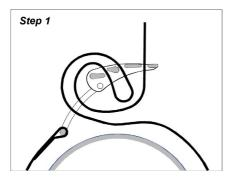
Pass the end through the end slot from back to front
