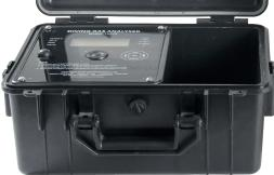
The analyser has the capability within the PCB to monitor helium, carbon monoxide and carbon dioxide.
